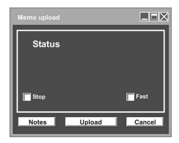
**Upload** Starts the data transmission from the instrument to the PC.
